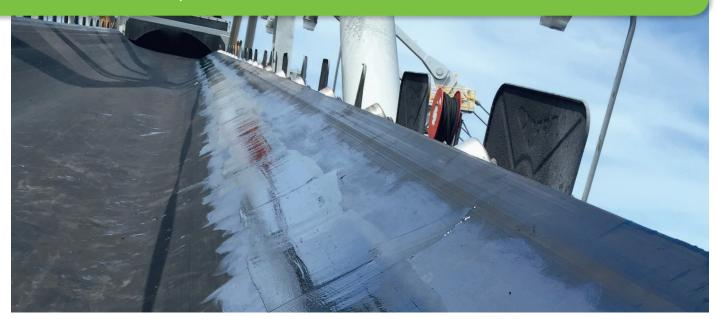
Qik Fix is a two-part 100% solids polyurethane repair kit used for the repair of rubber (fabric and steelcord), Nitrile and PVC conveyor belts and linings.
